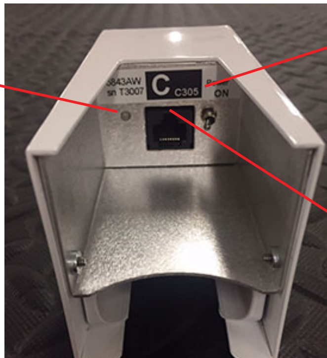
Figure 1 - T-Link3 power and external connections
