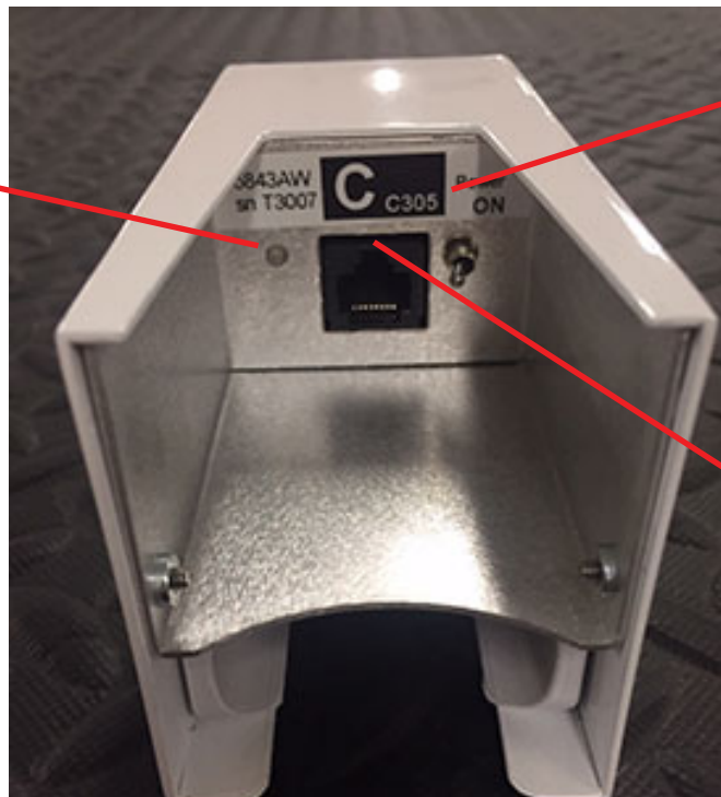
Figure 2 - T-Link 3.0 power and external connections
