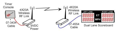
A 2800 Series RaceAmerica XL Professional Timer sending data to a Scoreboard with RS422 Red connections Timer to Wireless and RS232 Blue connections Wireless to scoreboard.
