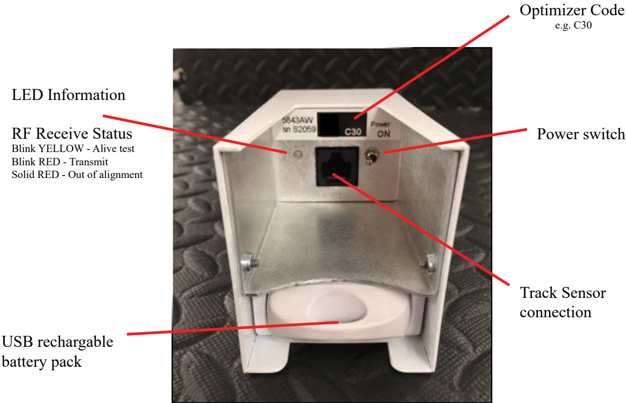
Figure 4 - T-Link 3.0 power and external connections
