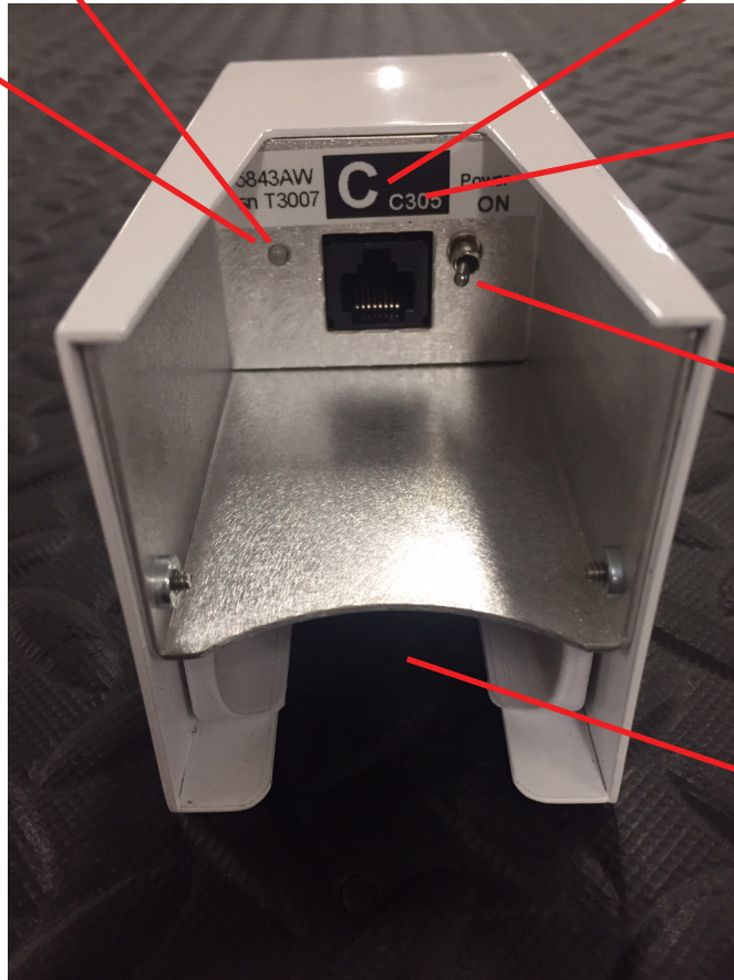
Fig. 6 - T-Link control center. The track sensor cable plugs into the T-Port connector.
