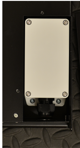
Figure 3 Exposed Power Box with rear panel removed.
