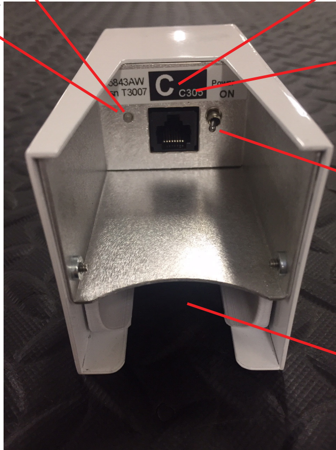
Fig. 3 - T-Link control center. The track sensor cable plugs into the T-Port connector.
