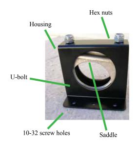
MOUNT COMPONENTS - The mount package contains one U-bolt with two nuts, one U-bolt saddle, one housing and four #10-32x0.375" stainless steel screws.
