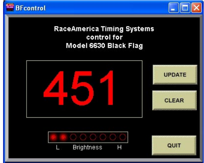
Figure 5 - Dimming - click and drag dots on brightness bar to control brightness of display.
