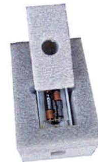
Installing a 5040 Emitter Similar for 5140 Sensor
