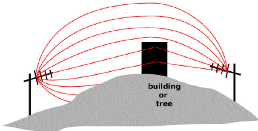
Because of the combination of signals being received and the angle of phase shift between them, the antenna position may need to be adjusted. In this application of a wireless link, the direction the receiving antenna is aimed may not relate to the location of the transmitting antenna, but more relates to reception of the 'best combination' of reflected Fresnel Zone signals.
