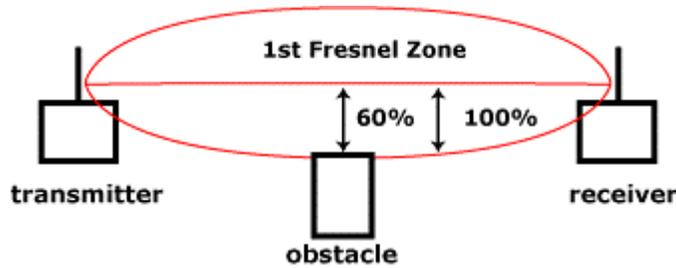
Since the 1<sup>st</sup> Fresnel Zone is closest to the direct path signal, the general ‘rule of thumb’ is to maximize 60% of the 1<sup>st</sup> Fresnel Zone by avoiding obstacles between the transmitter and receiver. Raising the antennas can increase the amount of the direct signal received by decreasing the amount of good signal blocked by an obstacle in the 1<sup>st</sup> Fresnel Zone.
