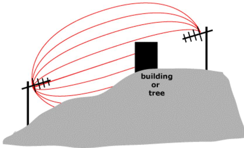
A pair of Yagi type antennas installed at the bottom and top of a hill is used to focus the radio waves. Raising the antennas may not be all that it takes since obstacles like buildings and trees may block the direct path signals leaving only the other Fresnel Zones to establish a link between antennas. This may require more transmitter power than the direct path signals but it will work
