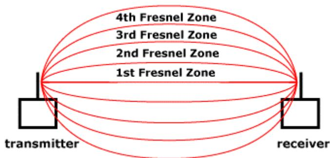
Signals received through the zones 1, 3, 5, etc. have more negative effects on the wireless communications while signals received from zone 2, 4, 6, etc. can actually have positive effect on the wireless connectivity. This is all due to the phase shift occurring at different ‘angles’ when compared to the direct line signal. If the receiver receives enough phase canceling signals, the total could cancel out the direct path signals resulting in signal loss.
