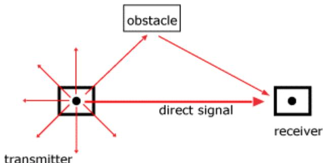
Being able to see the receiving antenna (line-of-sight) does not guarantee the wireless link will establish and operate properly. Radio waves do not travel between the transmitter and the receiver in just a straight line. For standard ‘Rubber Duckie’ type omni-directional antennas, radio waves travel from the transmitter in every direction outward from the antenna.
